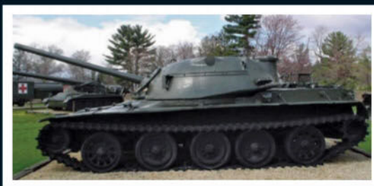
Right: The experimental T95 medium tank was the first to utilise composite armour
